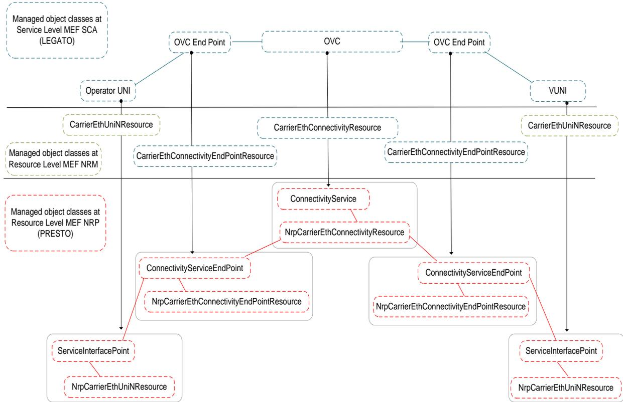
**Figure 18-MEF 7.3<sup>1</sup> Operator UNI/VUNI/OVC/OVC End Point-to-MEF Presto NRP Mapping**
