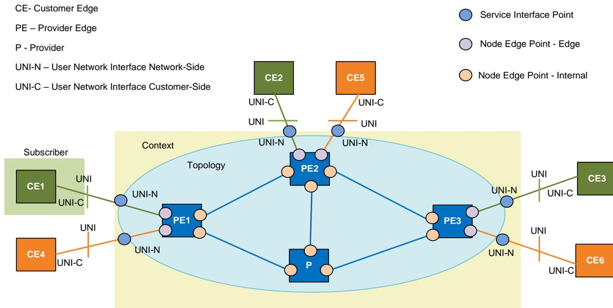
**Figure 13-Simple network example to illustrate ONF TAPI Topology**
