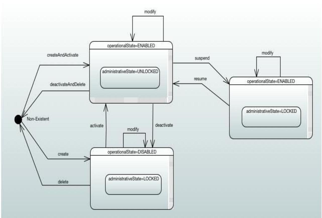
**Figure 40-Connectivity Service End Point State Machine**
