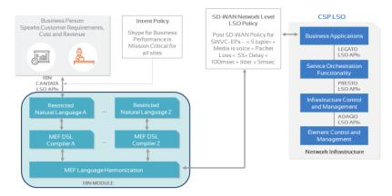
Figure 19 - Using Intent-Based Networking for SD-WAN services
