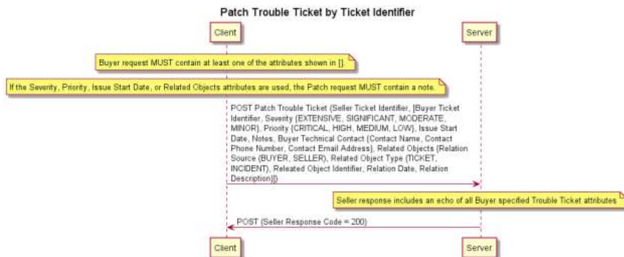
Figure 63 – Patch Trouble Ticket by Ticket Identifier Sequence Diagram
