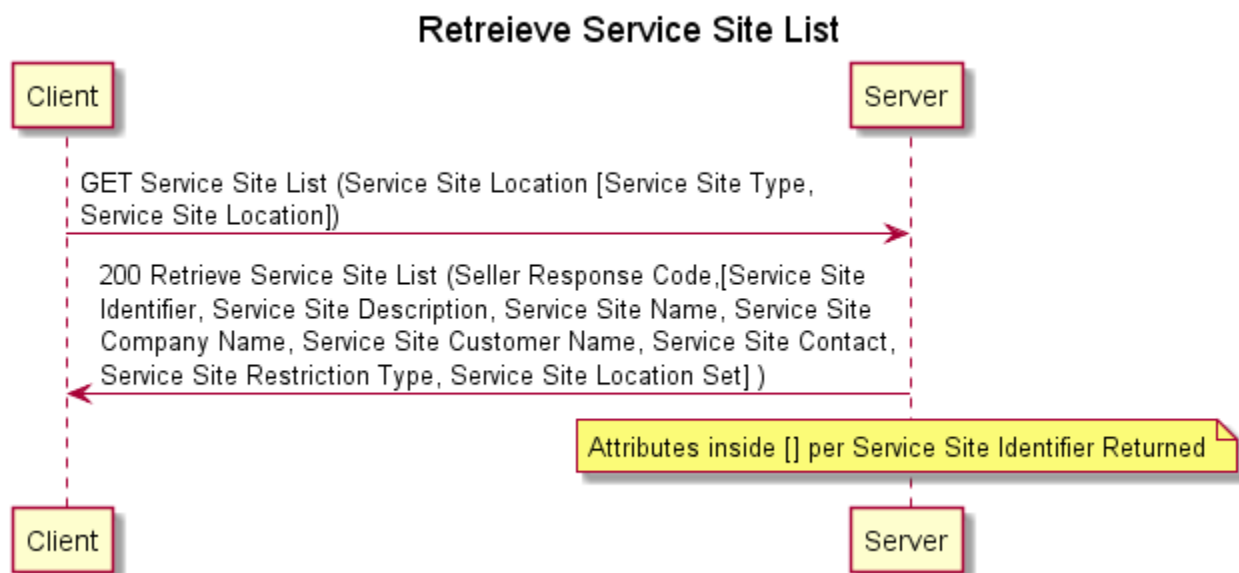
Figure 6 – Retrieve Service Site List Sequence Diagram
