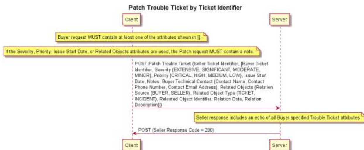
Figure 66 – Patch Trouble Ticket by Ticket Identifier Sequence Diagram
