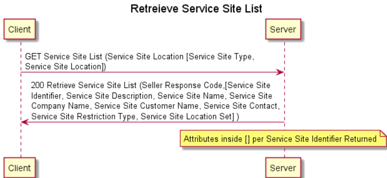
Figure 6 – Retrieve Service Site List Sequence Diagram
