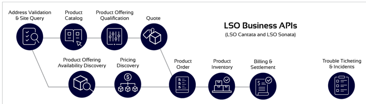
Figure 3. Cantata and Sonata End-to-End Function Flow
